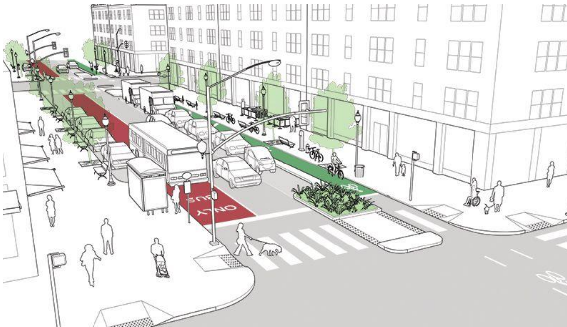
An example from NACTO Complete Streets showing improved urban streetscapes with tree canopies, a high frequency bus lane and wide footpaths for improved amenity.
