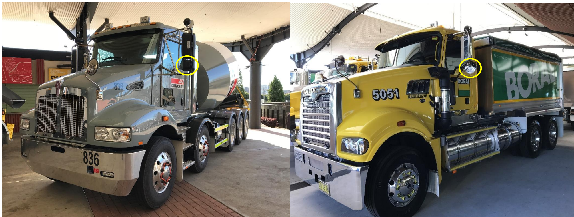
Figure 4.6 Examples of Class IV mirrors
