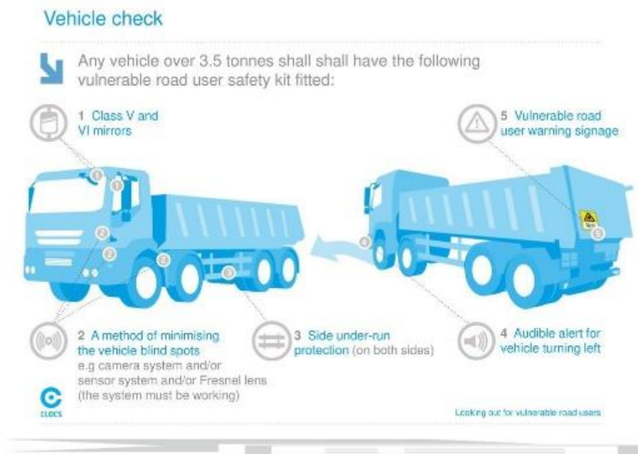
Figure 3.1 Overview of VRU related safety technologies that should be fitted to heavy vehicles 23
