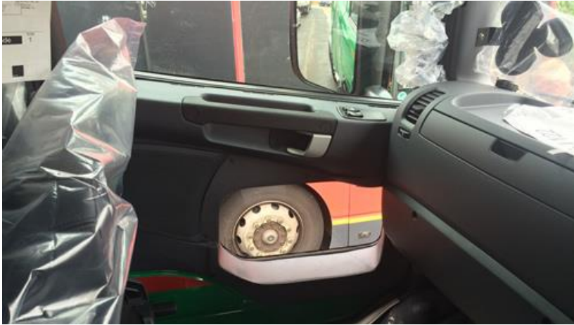
Figure 4.11 Example of truck door direct vision window 34
