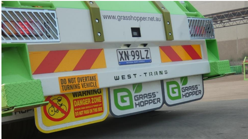
Figure 4.13 Examples of rear warning signage - Image courtesy of Sydney Metro.
