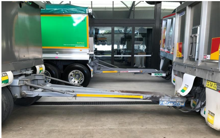
Figure 4.16 Example of stripe marking on trailer bar - Image courtesy of Sydney Metro.
