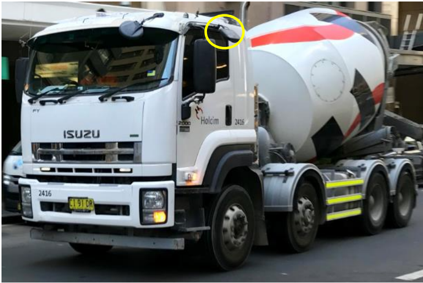
Figure 4.7 Examples of Class V mirrors 27
