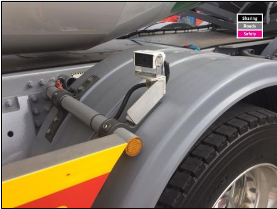
Figure 4.9 Example of blind spot camera on the outside of truck 33
