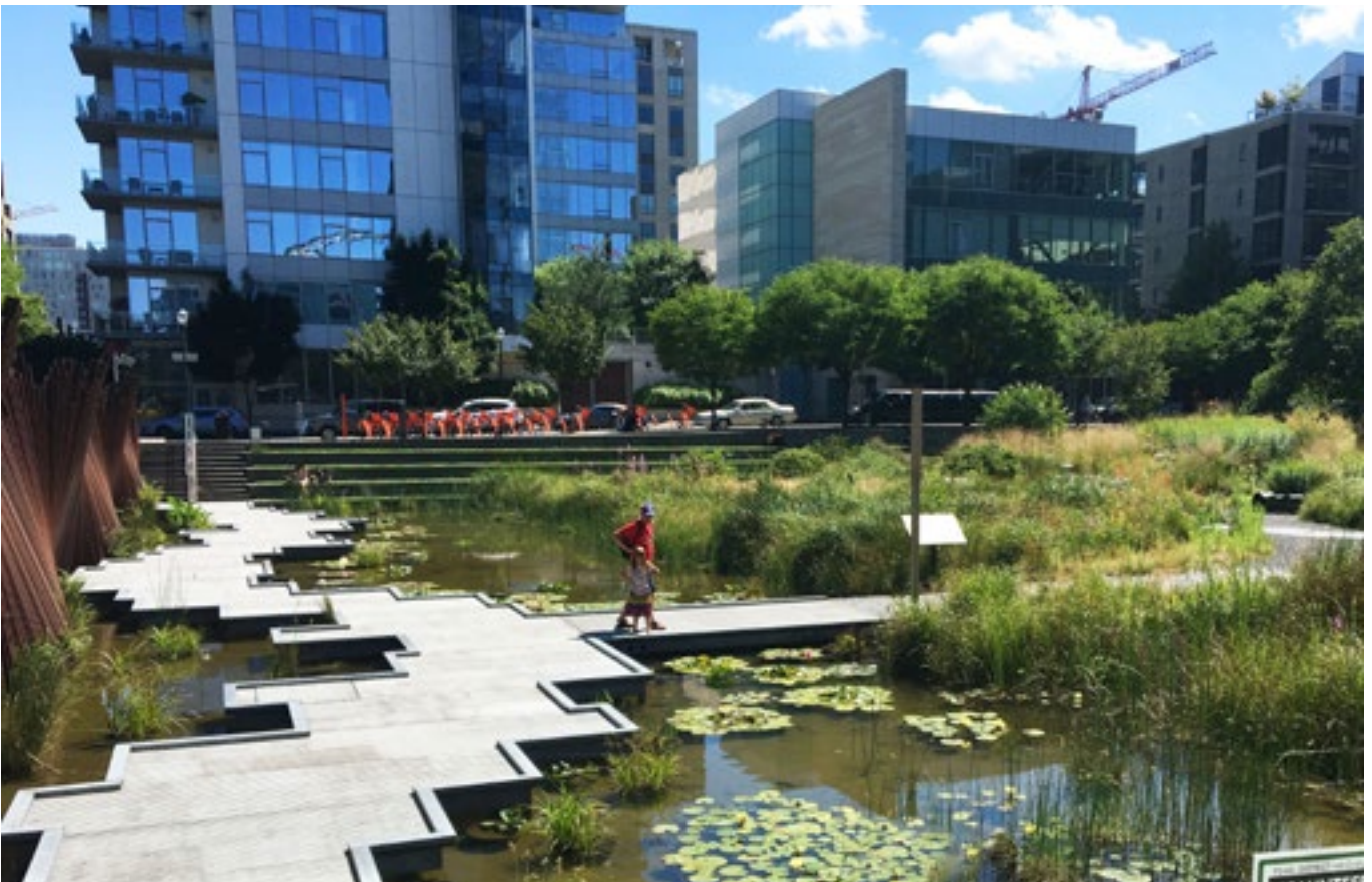
Figure 50 Example of an open space in Portland, Oregon which also manages stormwater during flood events
