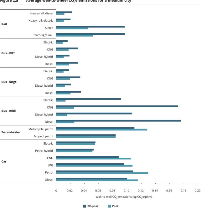
Figure 2.5 Average well-to-wheel CO<sub>2</sub>e emissions for a medium city
