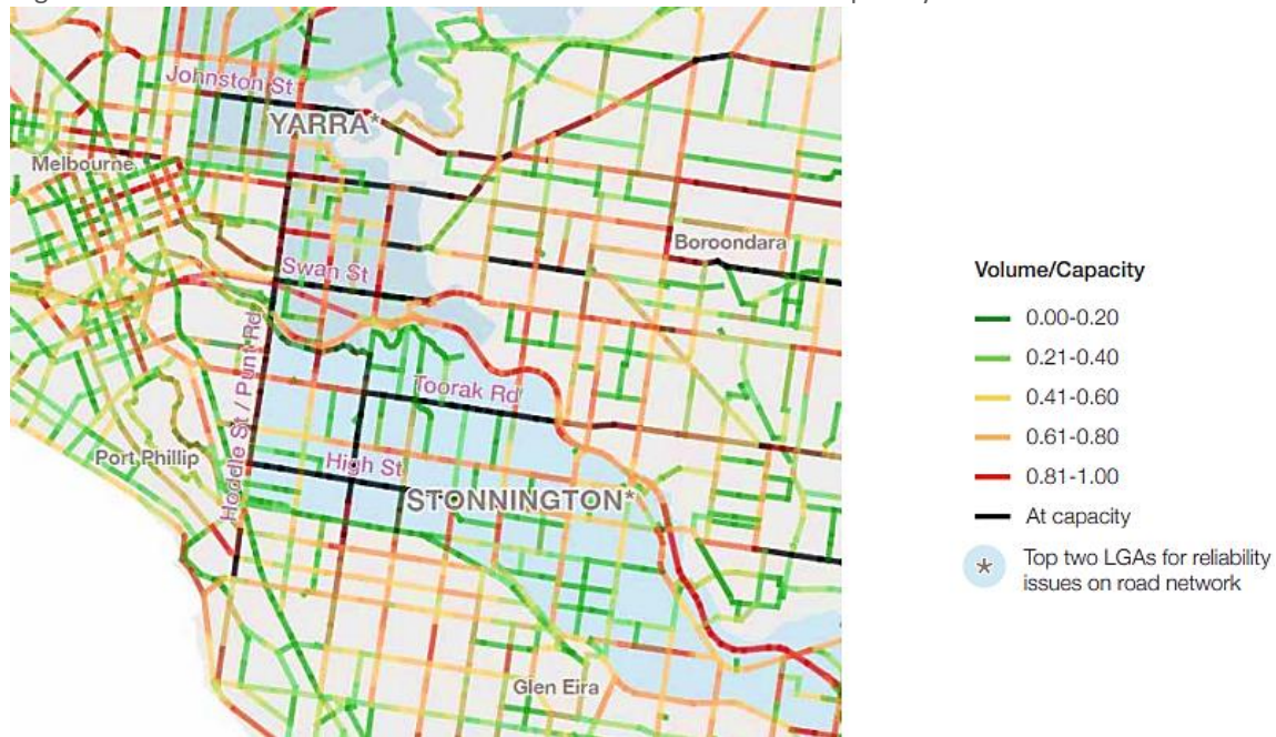
Figure 5: Areas where volume of traffic nears or exceeds capacity of the roads
