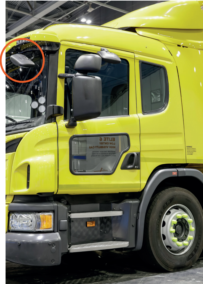
Class VI mirror shall be fitted to the front of the vehicle
