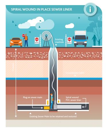
The technique we are using to upgrade the sewer is called 'relining'. This involves unwinding the relining material as a flat strip from a spool at the top of the manhole. The new plastic sleeve is wound into place, lining the inside of the existing sewer pipe. The gap between the existing pipe and new liner is then filled with cement (called grouting).
