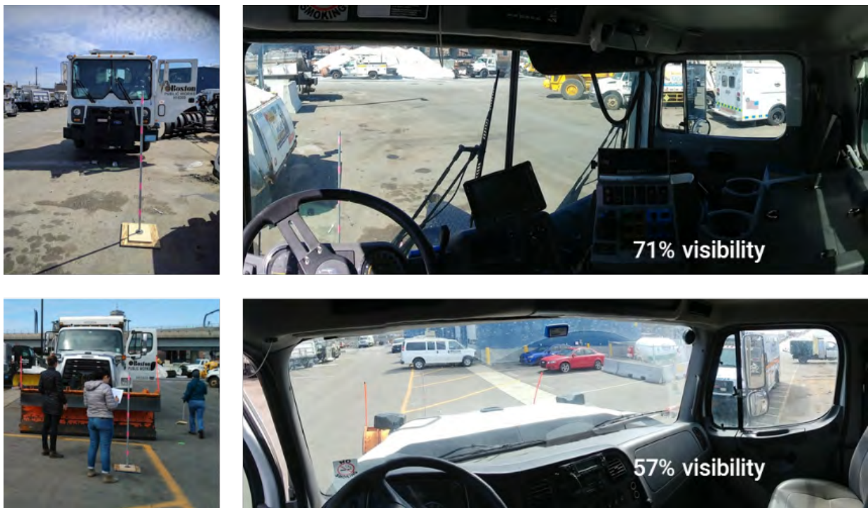
Figure 21: Comparing direct vision of a cabover and conventional cab truck using the VIEW method.
