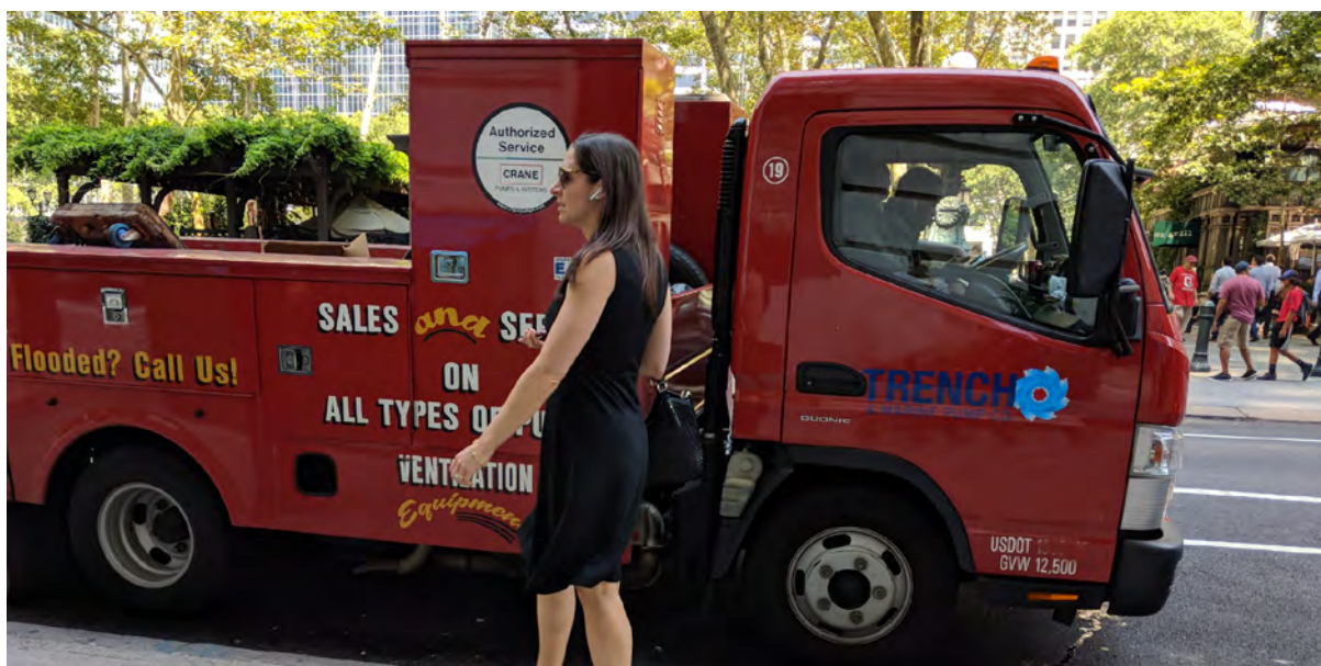
Figure 10: The Mitsubishi Fuso Canter, pictured here in New York City, features a low-entry, reduced height cab which increases the driver’s ability to see people and objects.
