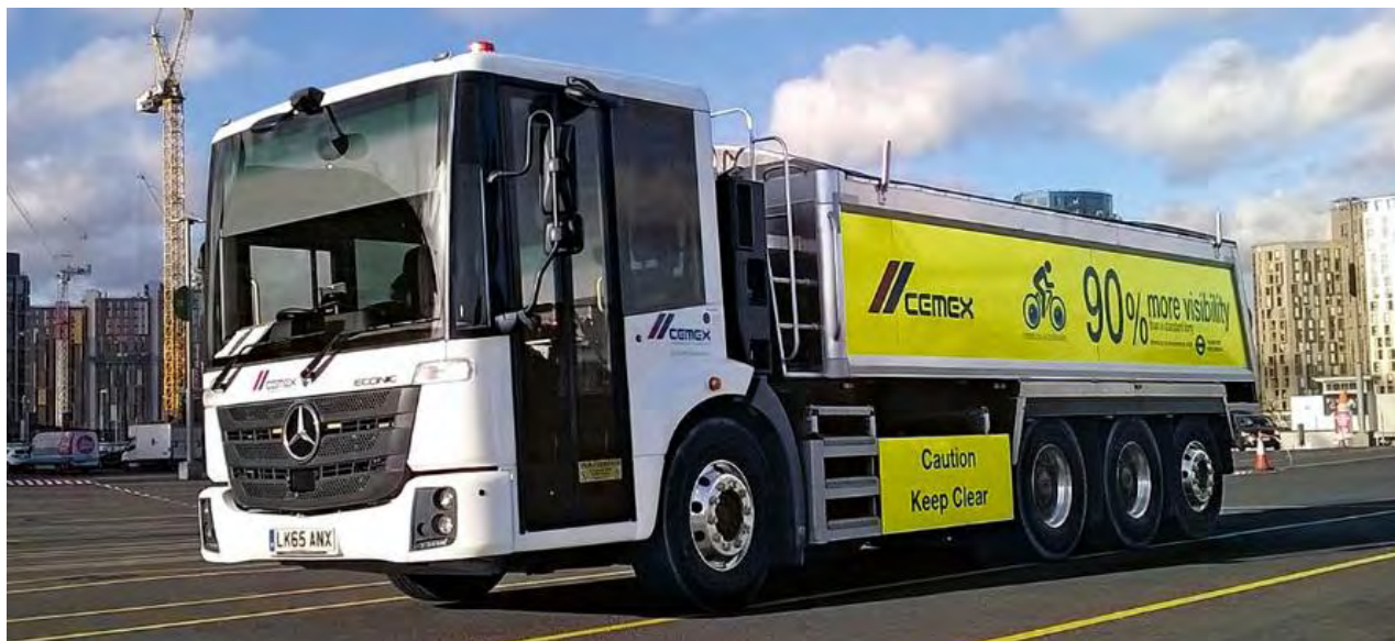
Figure 7: This CEMEX dump truck, used to supply sand and gravel to London concrete plants, features a high-visibility cab and cameras and radar side sensors to detect cyclists.
