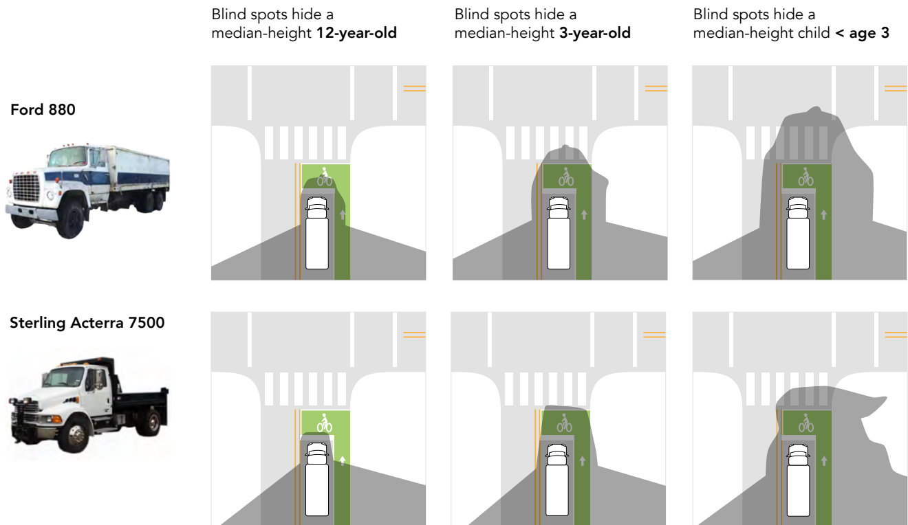
Figure 2: A vehicle with smaller blind spots better allows a median-height driver to see people in a bike box or a crosswalk, especially children. For the 50% of drivers who are below median height, the blind spots are actually larger than shown.
