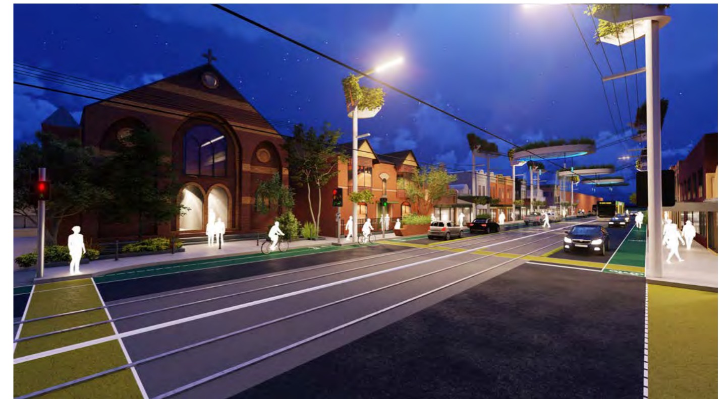
Figure 5. A hook turn bay allows cyclists seeking to turn right to safely wait for a dedicated green bike lantern sequence
