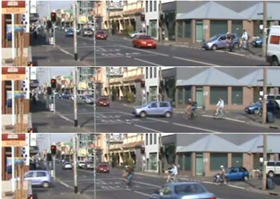
Figure 21 shows a pedestrian crossing away from the lights, forced to run to get across the road before the approaching car. After signalisation of the intersection, far fewer pedestrians were observed crossing in a gap, with almost all crossing at the designated pedestrian crosswalks and waiting for the green pedestrian signal.
