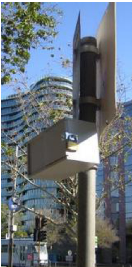
Fig. 1. Video camera box in position on a sign post.
