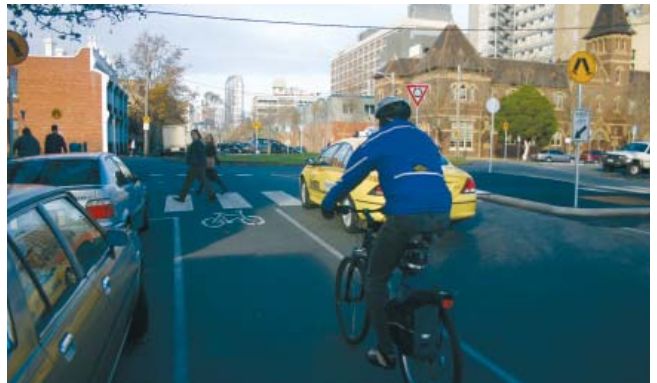
Figure 18 – Bicycle lane and pedestrian crossing at roundabout on Faraday Street and Cardigan Streets, Carlton
