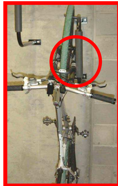
Straight design means that the forks rest on the rail, which may cause damage to bike and rail
