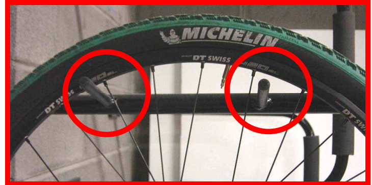
Bike is supported by lateral pressure on spokes, which may cause damage
