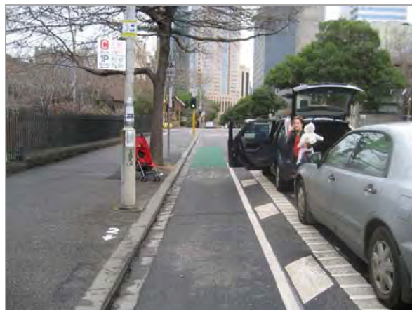
Buffer zones provide separation between the bike lane and the parking lane.
