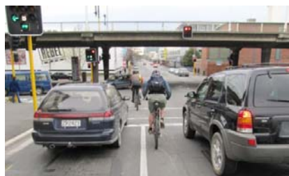
Bike riders, buses and left turning vehicles get a green before general through traffic at the intersection of Colombo St / Moorhouse Ave in Christchurch, NZ
